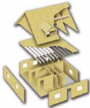
Supplied as fire rated and robust detail timber frame panels. Spandrel and gable panels make it possible for our clients to fully erect the entire roof structure in one operation; saving time, cutting costs, reducing scaffolding requirements and minimising the health and safety issues associated with building high gabled walls in blockwork.
