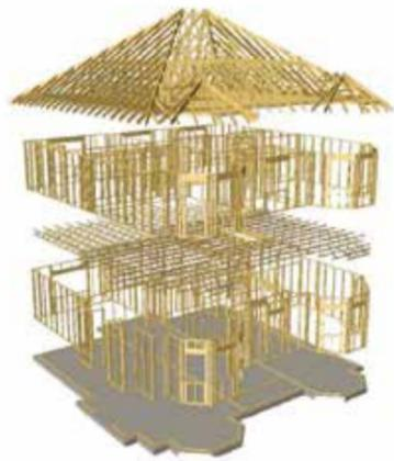
Applying modern design and manufacture methods to one of the oldest forms of construction allows us to produce exceptionally accurate, air tight, durable structures which meet the most stringent regulations with excellent performance characteristics.
