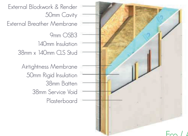
Eco / A2 U value - 0.14W/m 2 K Overall Width - 397mm
