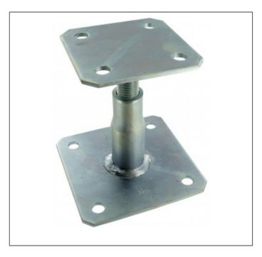
The APB features a post mounting plate on a screw allowing it to be adjusted to a specific standoff height ranging from 100-150mm. Suitable for post sizes 100 x 100mm to 200 x 200mm.
