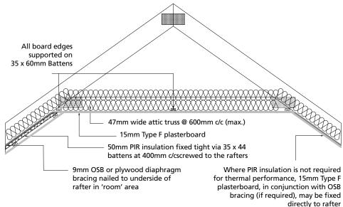
NOTE – All service penetrations [e.g. downlighters, soil vent pipes, ventilation duct heads, etc.] in the plasterboard create vulnerability in the ceiling and as such must be fire-stopped by the use of fire collars, fire hoods or fire-rated products.
